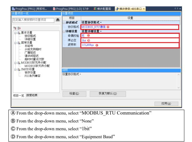
\*The communication format setting must be consistent with ID-GRID\*
